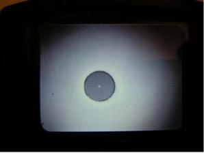
Check each connector face with at least a 200x power view scope to confirm that no imperfections are found.
